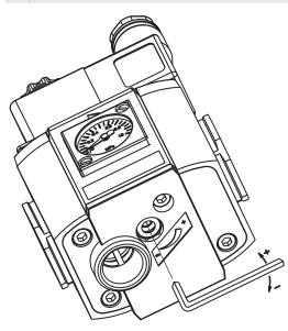
Manually adjust the "+" and the "-" throttle screw at the bottom of the soft start-up valve as per the requirement of start speed. It shall go slowly, otherwise sudden acting of the product or system shall be caused with a heavy impact.
